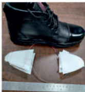
Position of TENG inside the sole
