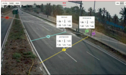
Live highway view with vehicle count and classification displayed.
